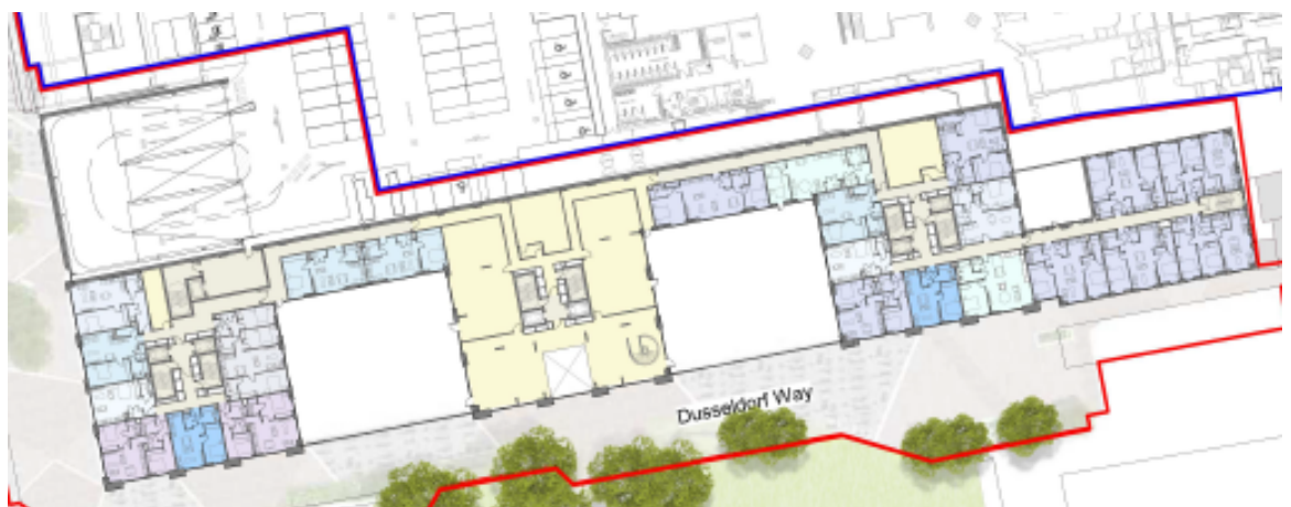
Layout of accommodation, Level 01 (car park roof level)
